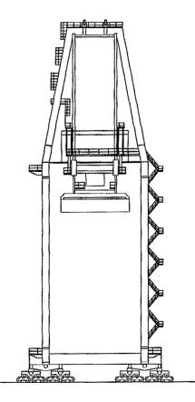
B-1.8 **Locomotive Cranes.** Locomotive cranes are used for railroad service applications where access by other cranes is not practical or desired.
