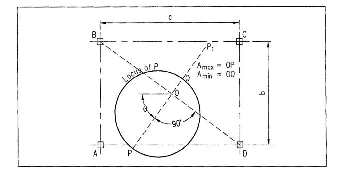
Figure B-21 Relative Variation of Corner Load During Full Rotation
