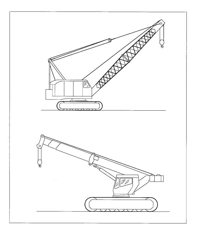
Figure B-18 Mobile Cranes (Crawler Mounted)
