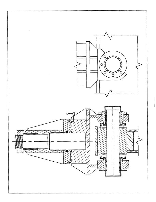
2-2.12.1 **Rocker Pins.** Cranes that travel on straight tracks do not require gudgeons. The rocker motion is provided in the form of rocker pins and reinforced extensions of the webs or saddles, either upward or downward, at the pivot points.
