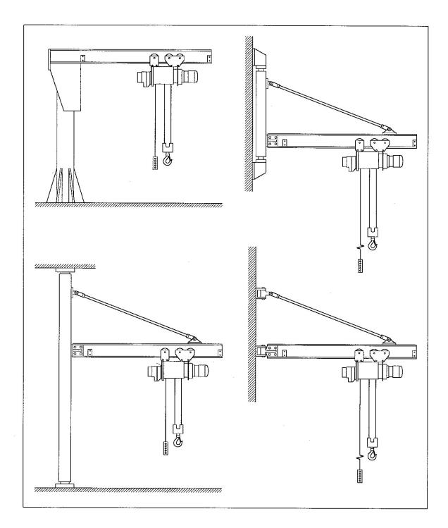
Patented track booms are available by specific request at additional cost; however, the booms on these cranes are most often in the form of single-web girder. The hoist is typically an under running hoist/trolley unit. The individual motions may be electrically driven and controlled from a pendant pushbutton station or manually operated.
