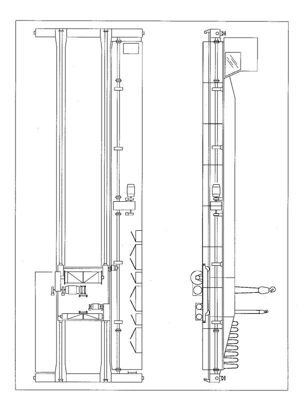
B-1.1.2 **Distinctive Features.** The stable platform of the bridge structure of top running bridge cranes permits a wide range of design options to suit virtually any operational requirement. The high overhead location of these cranes avoids interference with the floor activity and equipment by lifting the loads over the floor obstructions. Walkways along the bridge girders and the floor on the trolley structure provide excellent accessibility to mechanical and electrical components.
