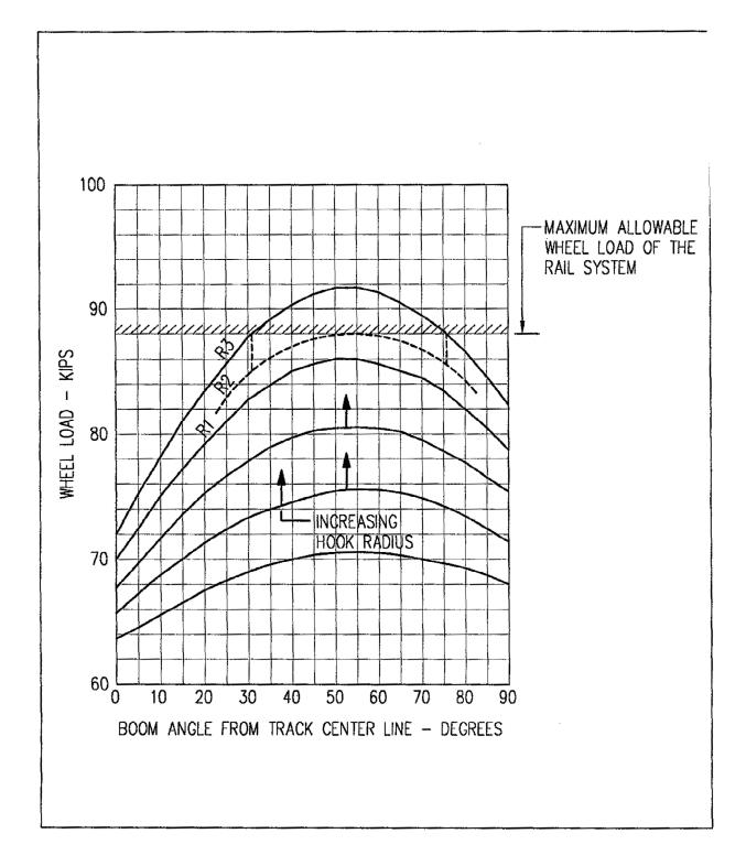
Figure B-19 Variation of Wheel Load Through a Quadrant of Rotation
